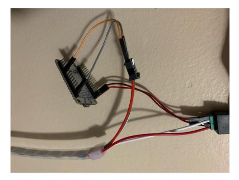
There were many possible choices, but for the current implementation the generic ESP8266 microcontroller is sufficient as this board is capable of handling 5 volts and also has the necessary onboard pins we require: ground, vin, and data - it also has others, which may be used down the line for more advanced features. Above is a photo of our current hardware implementation, excluding the power supply.
